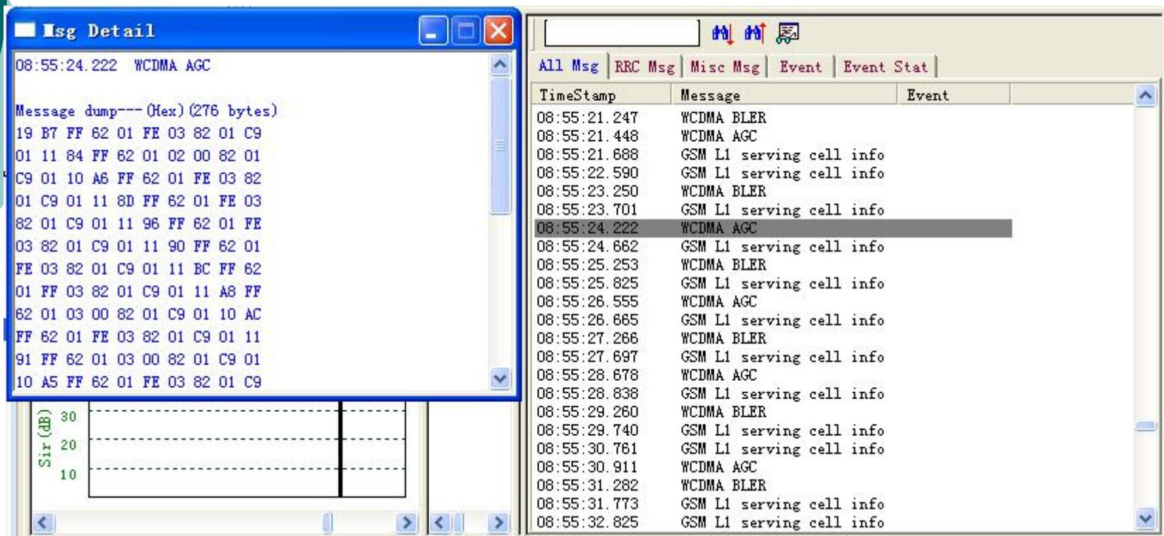
Complete air interface signaling acquisition and decoding.
