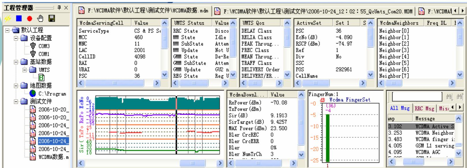
Designate a WCDMA/GSM mobile phone in the region and around the NodeB then record the procedure between the cell phone and Node B which include channel Switching, station switching, disconnection etc. It will be helpful to understand the problem.
